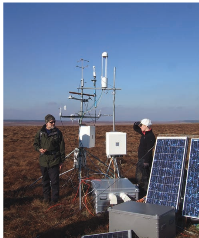
Figure 1.2 A flux tower on a peatland which can be left to run automatically. The instruments on the tower are used for measuring the uptake and release by the landscape of CO 2 , energy and water vapour.
